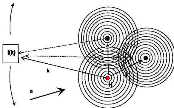
Figure 1. The monochromatic incident neutron beam illuminates the sample. Neutrons incoherently scattered by hydrogen nuclei form spherical waves. These waves partly are scattered by neighbouring nuclei and partly reach the detector located at large distance. The detector moving over a sphere around the sample records the interference pattern of these waves.
